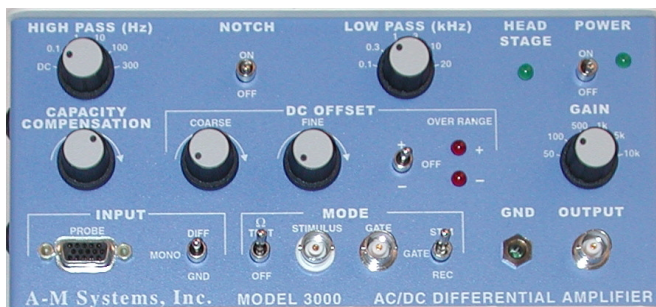
Figure NB-7-3: The front panel of the Model 3000.
