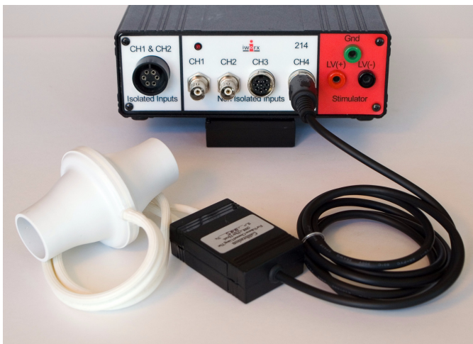
Figure HS-1-2: A SP-304 spirometer connected to an IWX/214 unit.
