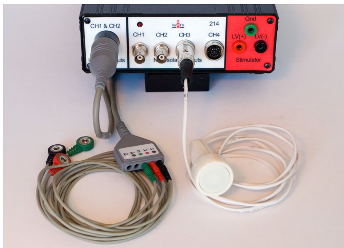
Figure HH-2-3: The ECG cable and event marker connected to an IWX/214.
