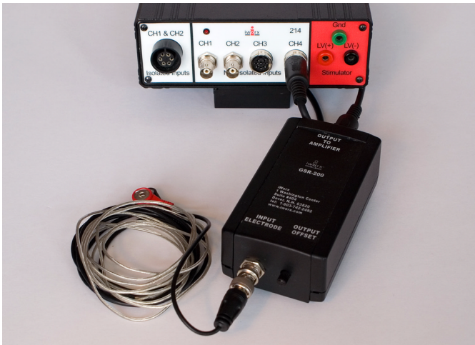
Figure HP-3-2: The GSR-200 connected to an iWX214.
