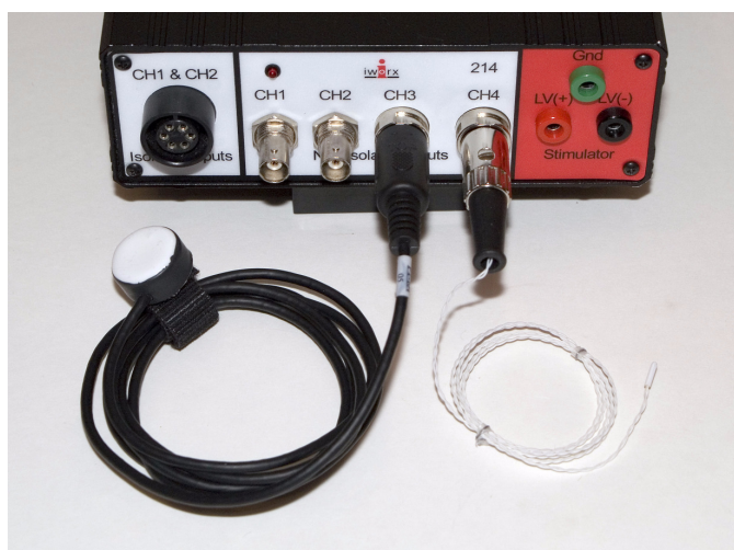
Figure HE-1-3: The PT-104 pulse plethysmograph and the TM-104 temperature probe connected to an iWorx/214 data recorder.
