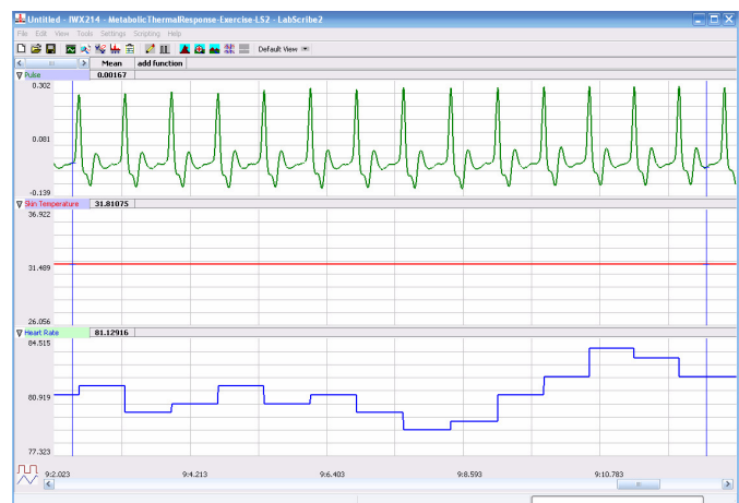
Figure HE-1-8: Pulse, skin temperature, and heart rate recordings while subject is at rest, displayed in the Analysis window.
