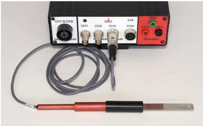
Figure FB-1-2: The FT-104 force transducer connected to the IWX/214.
