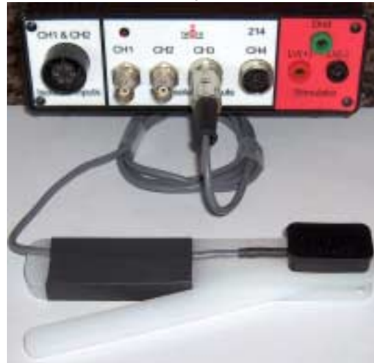
Figure HM-5-2: The GN-100 goniometer connected to an IWX/214.
