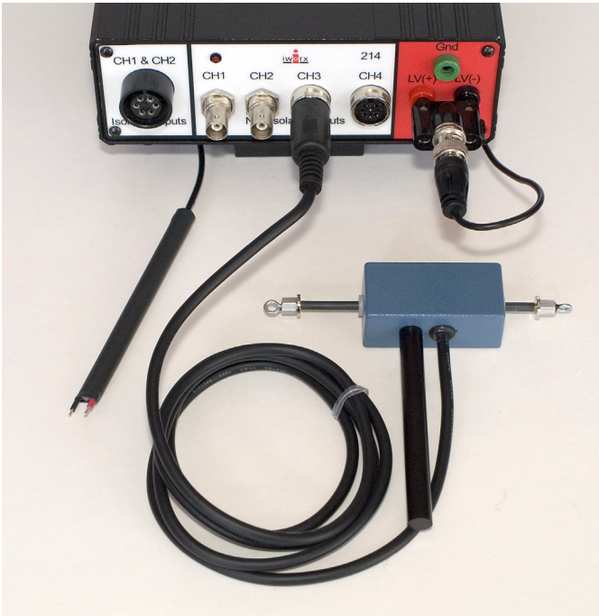
Figure AM-1-4: The DT-475 displacement transducer and the A-BST-100 bipolar stimulating electrode connected to the IWX/214.
