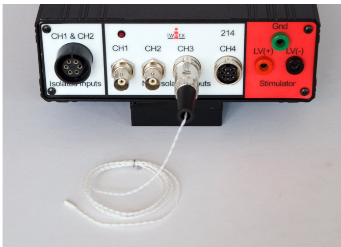
Figure HP-4-2: The TM-100 temperature probe connected to an IW214.
