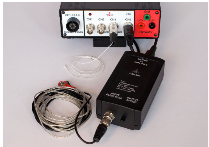
Figure HP-4-7: The TM-100 and GSR-200 connected to an iWX214.
