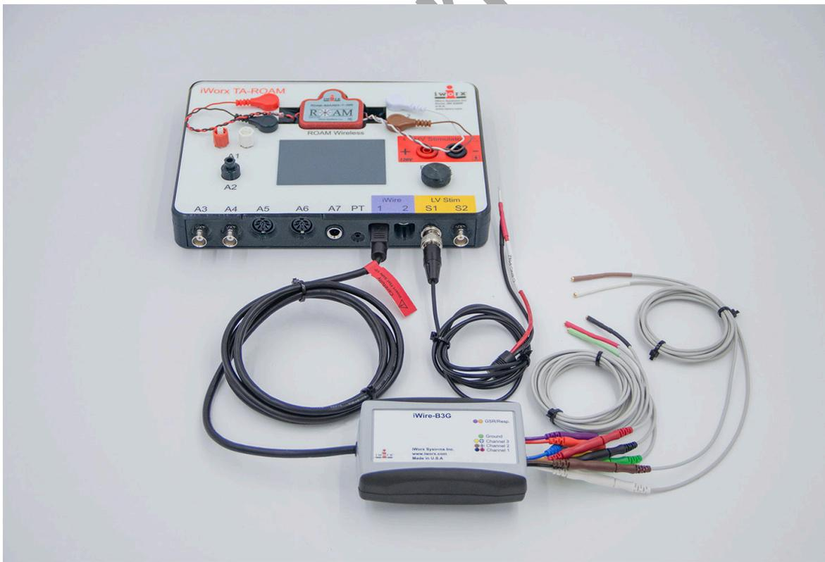
Figure AN-4-S1: The iWire-B3G recording cable and stimulator cables attached to the IXTA.
