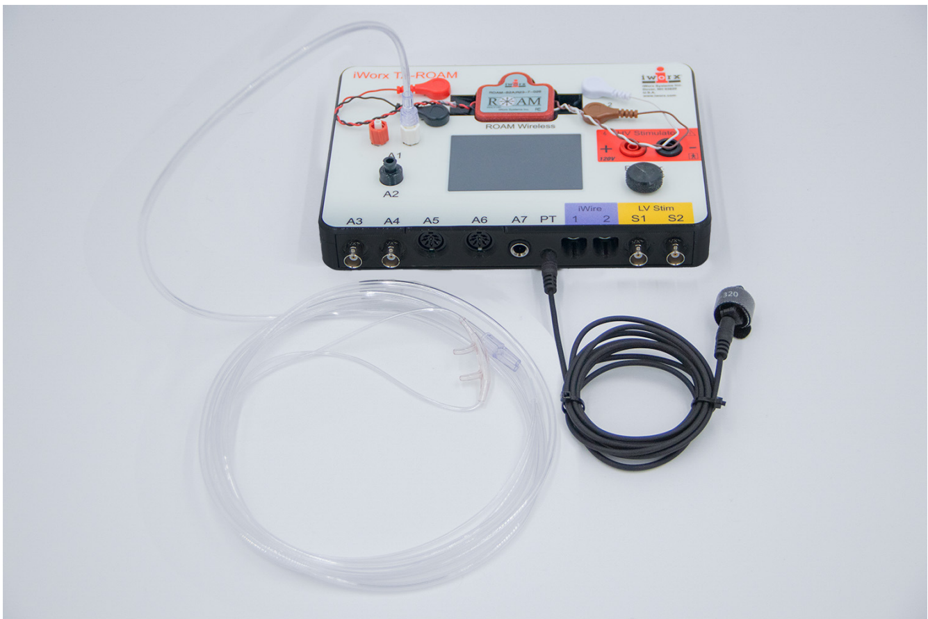
Figure HP-22-S2: TA showing the pulse/temperature sensor and nasal cannula set up.
