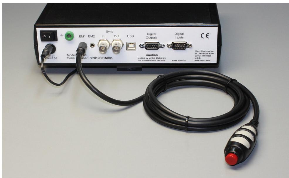
*Figure HN-1-S2: The IXTA with the EM-220 event marker.*
