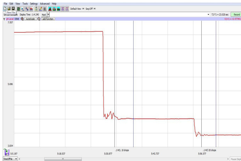
Figure GB-1-L1: Recording of the change in pH of the water when HCL is added.
