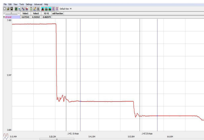
Figure GB-1-L2: pH recording in the Analysis window showing the pH values for the addition of 0.1M HCl to the deionized water.
