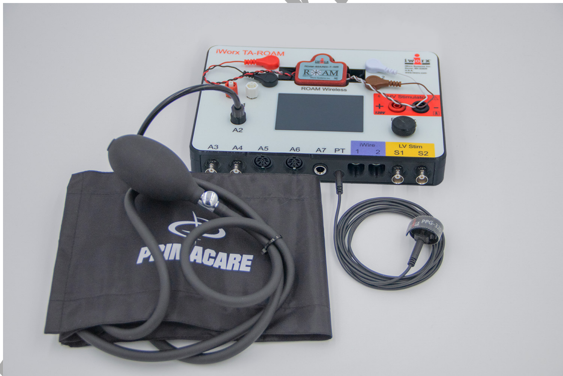
Figure HC-2-S4: The PPG-320 pulse sensor and the BP-220 blood pressure cuff connected to the TA.
