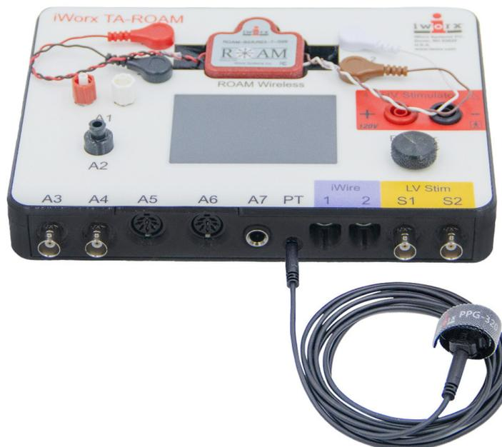
*Figure HS-5-S1: The PT-104 pulse plethysmograph.*
