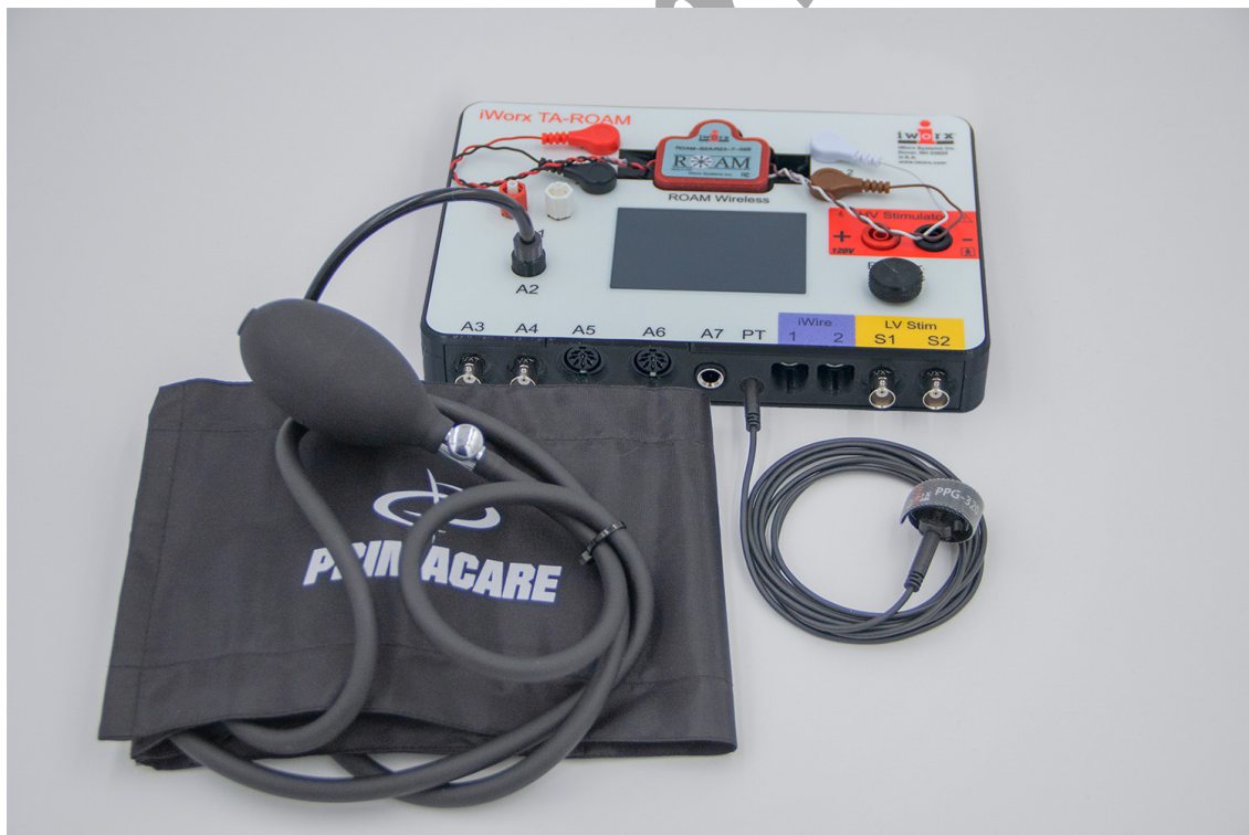
Figure HC-5-S4: The PPG-320 pulse transducer and the BP-220 non-invasive blood pressure transducer connected to the TA.
