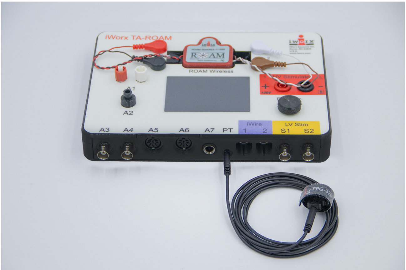
Figure HC-5-S2: The PT sensor plugged into the PT port of the IX-TA-ROAM
