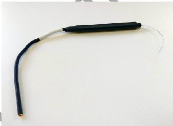
*Figure AN-7-S2: Monopolar extracellular hook electrode.*
