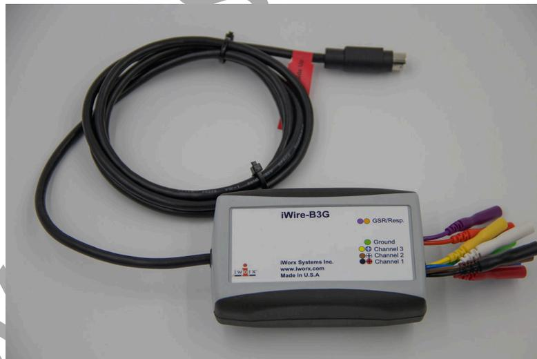
Figure AN-13-S1: The iWire-B3G recording cable.
