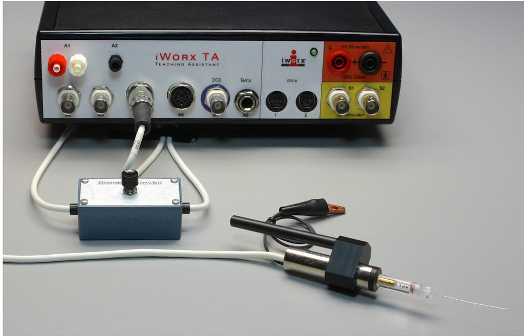
Figure AN-12-S5: The IC-200 intracellular probe with a microelectrode holder connected to an IXTA.
