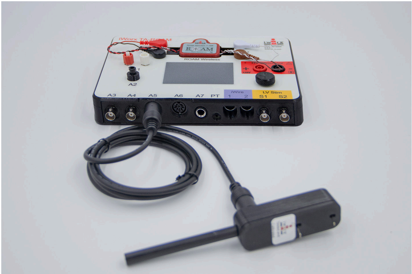
Figure AM-11-S2: The FT-302 force transducer connected to an IXTA.
