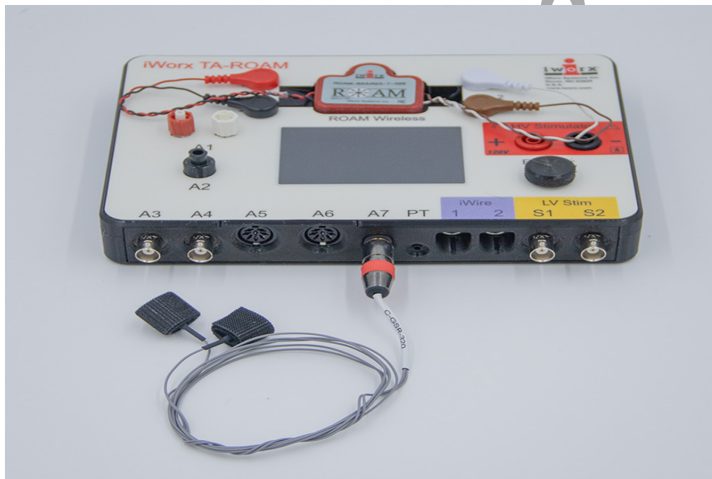
Figure HP-2-S1: The GSR galvanic skin response amplifier.
