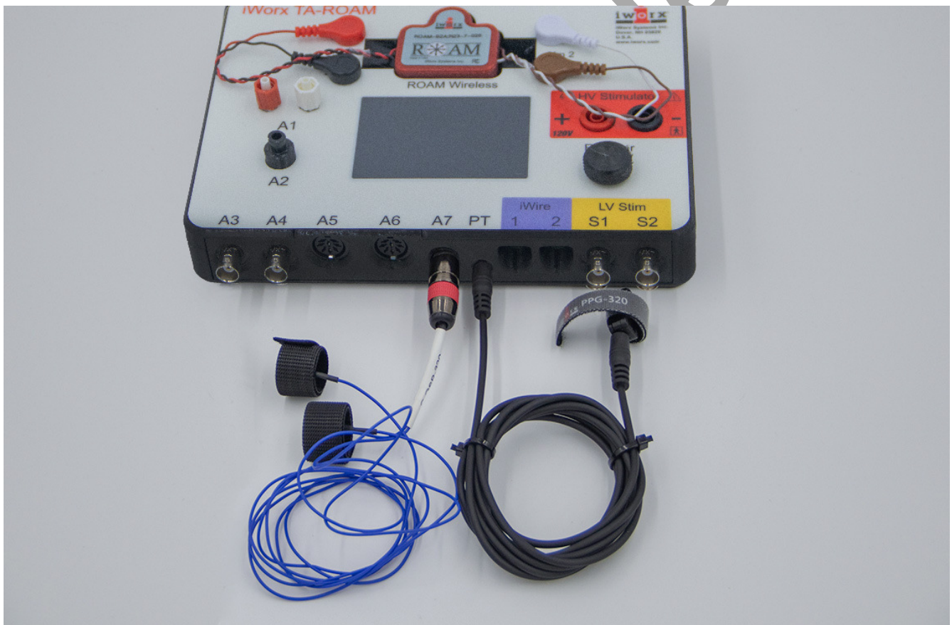
Figure HP-8-S2: The equipment needed to record GSR and pulse.
