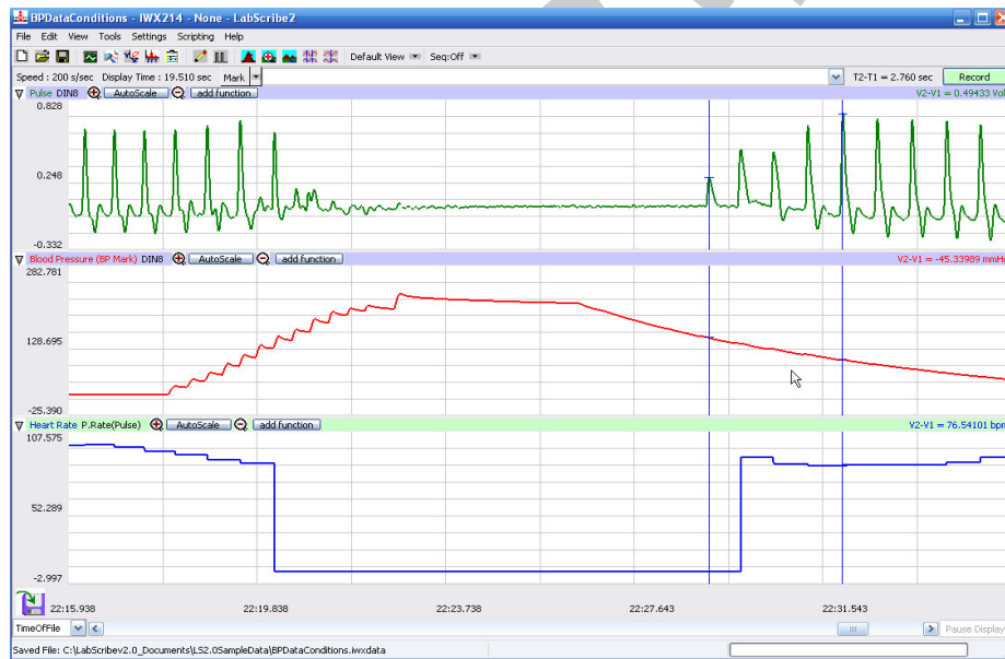
Figure HP-5-L2: The pulse waves and the pressure in the BP-600 recorded during the occlusion of the brachial artery as displayed in the Main window. Pulses disappear when the pressure in the cuff exceeds the pressure in the artery. The pulse wave reappears when the pressure in the cuff is released, The subject's heart rate is recorded on the bottom channel.
