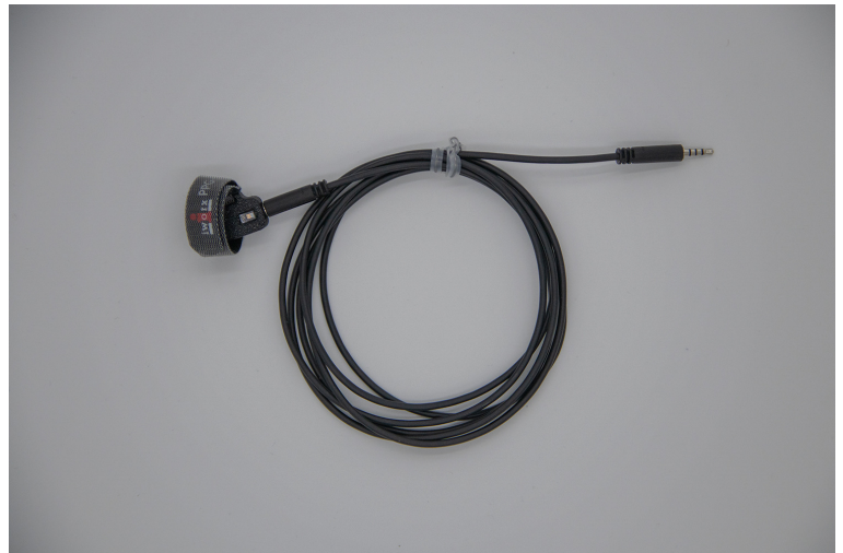
Figure HP-5-S1: The BP-220 non-invasive blood pressure transducer and PPG-320 pulse sensor.
