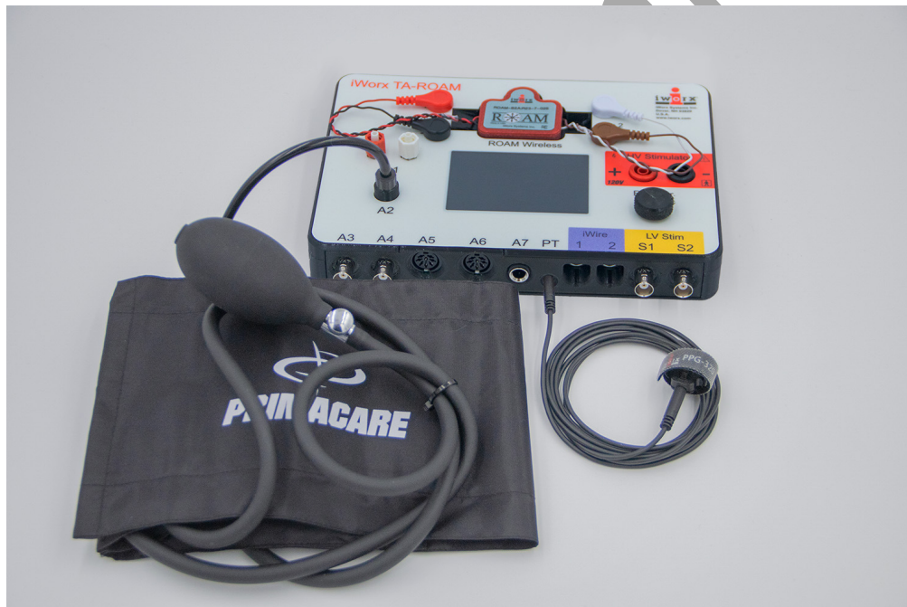
Figure HP-5-S2: The PPG-320 pulse transducer and the BP-220 non-invasive blood pressure transducer connected to an IXTA.
