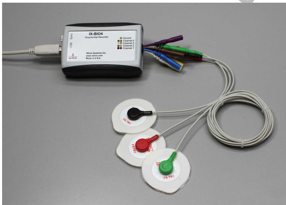
Figure HH-3-S1: The IX-BIO4 with three ECG lead wires and electrodes attached.
