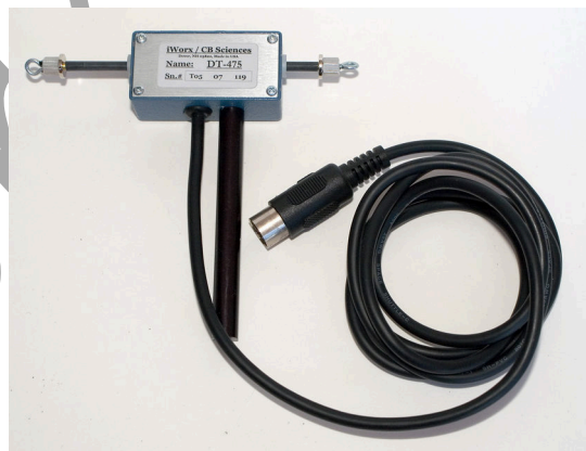
Figure AM-5-S1: The DT-475 displacement transducer.
