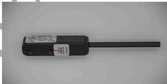
Figure AM-5-S3: The FT-302 dual-range force transducer.
