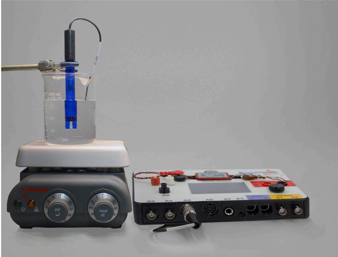
Figure GB-2-S2: The arrangement of the stirrer, pH electrode, and beaker for the calibration of the pH probe.
