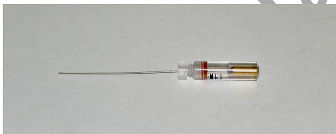
Figure AN-1-S2: The microelectrode holder for the IC-200.
