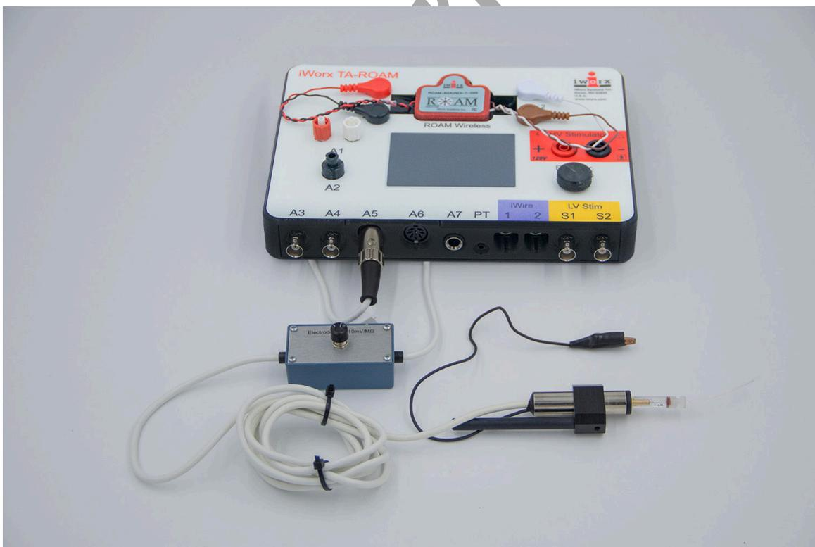
Figure AN-1-S3: The IC-200 intracellular probe with a microelectrode holder connected to an IXTA.
