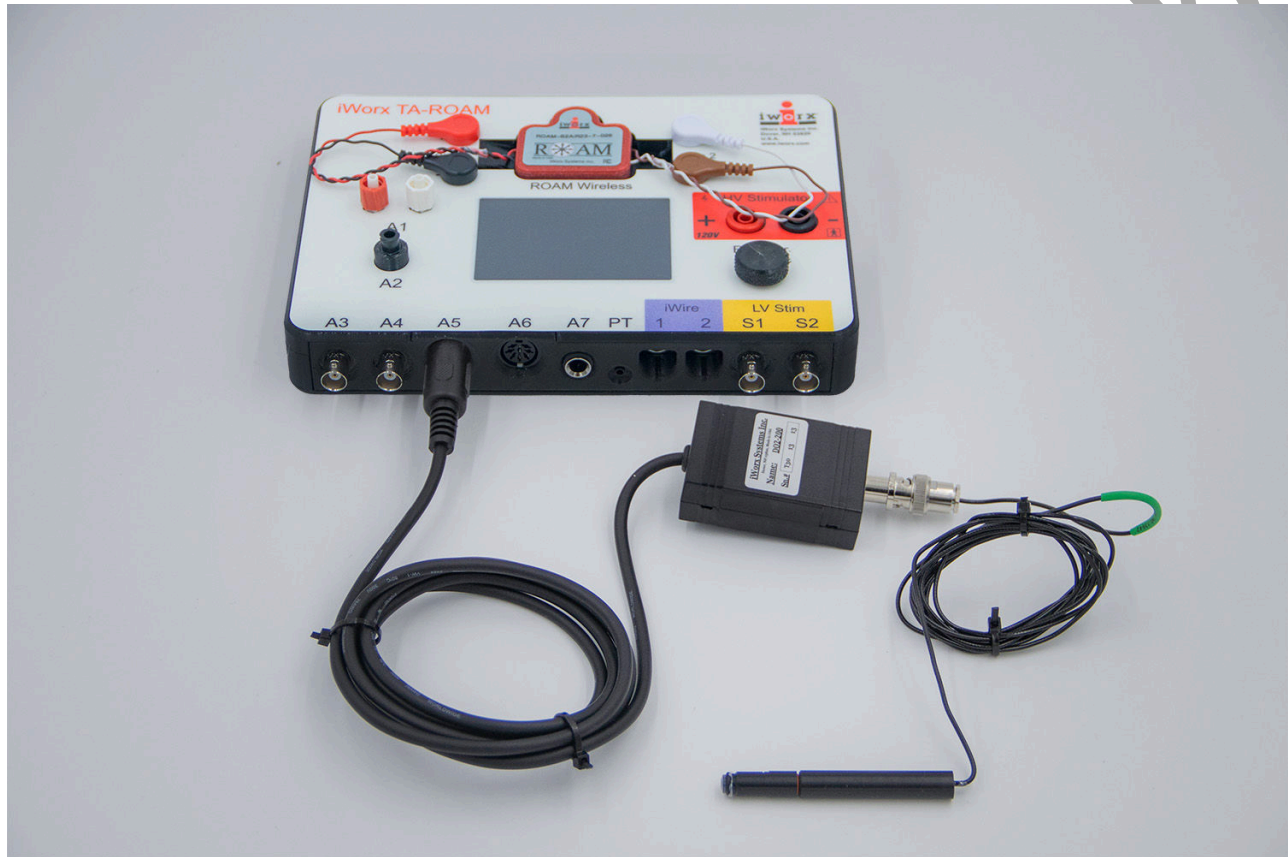
Figure CM-7-S1: Dissolved oxygen electrode connected to an IXTA.
