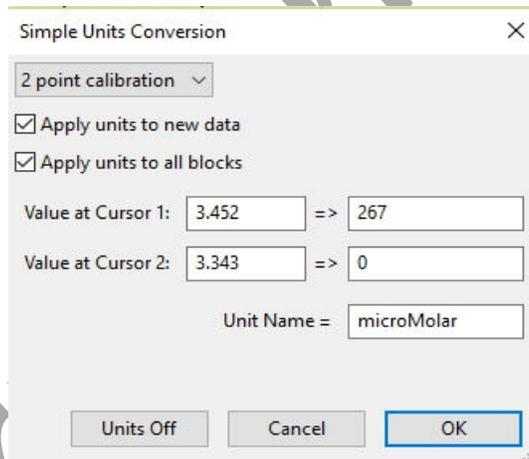
Figure CM-1-S4: The Simple Units Conversion dialogue window with the voltages at the cursors set to equal the dissolved oxygen concentrations used in calibration.
