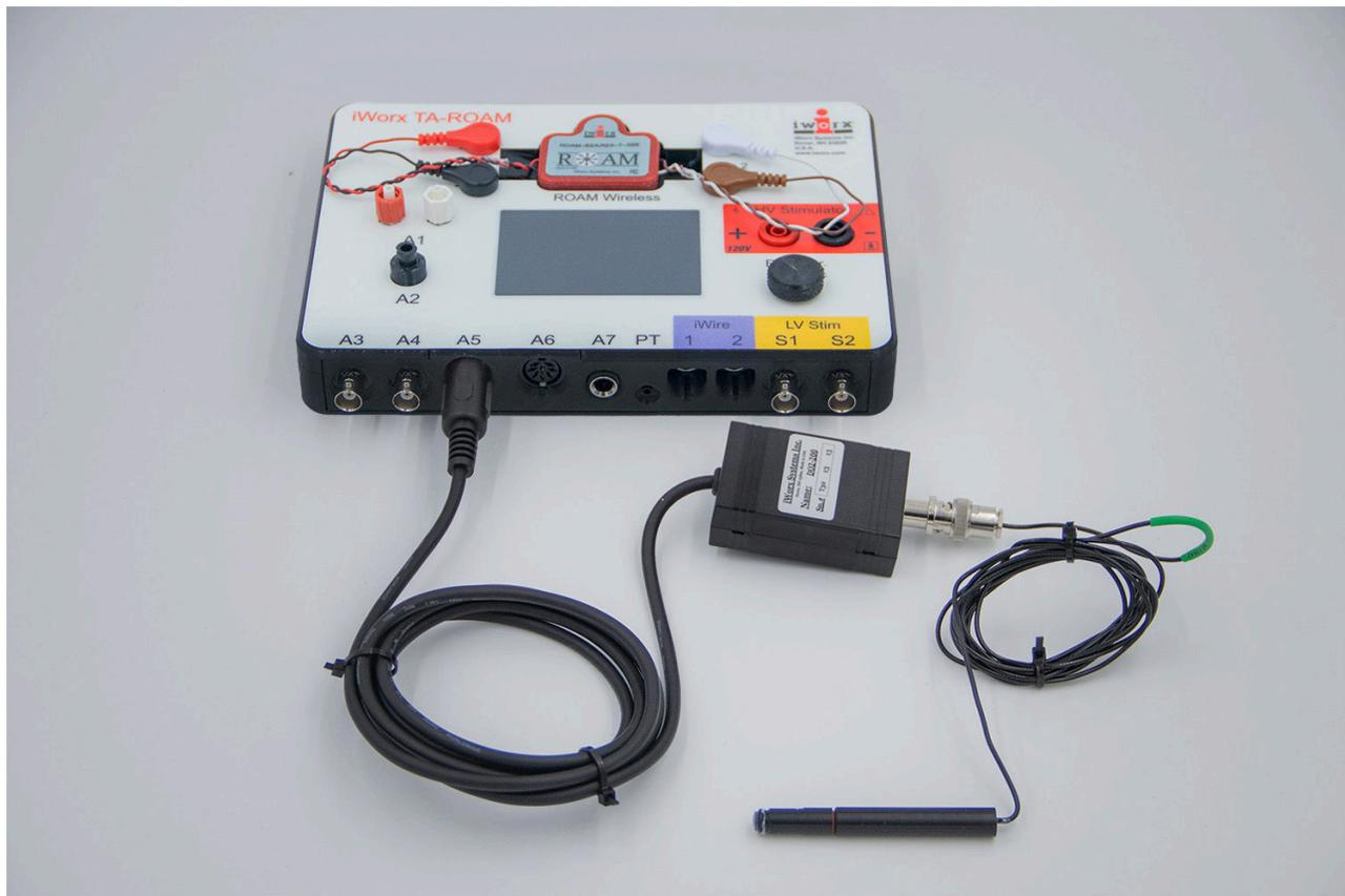
Figure CM-1-S1: Dissolved oxygen electrode connected to an IXTA.
