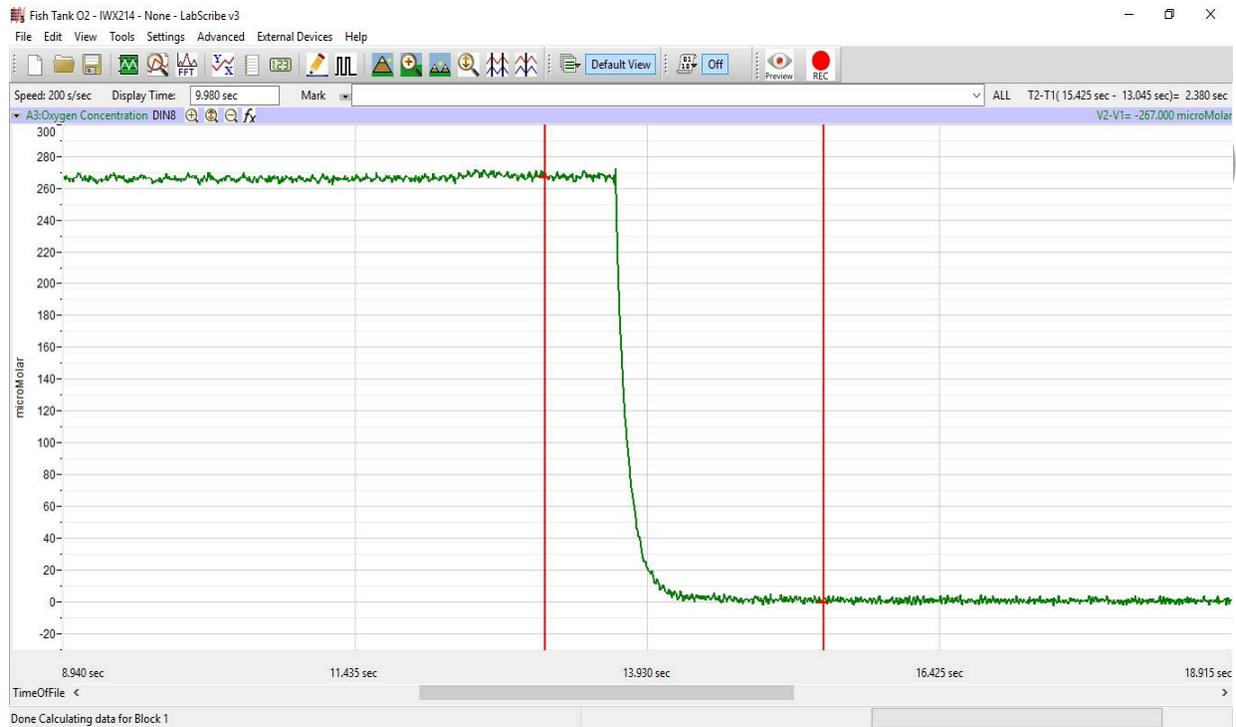
Figure CM-1-S3: Recording of oxygen concentrations in air saturated and oxygen depleted deionized waters used to convert the units of the Y-axis from voltage to  $O_2$  concentration ( $\mu$ Molar).
