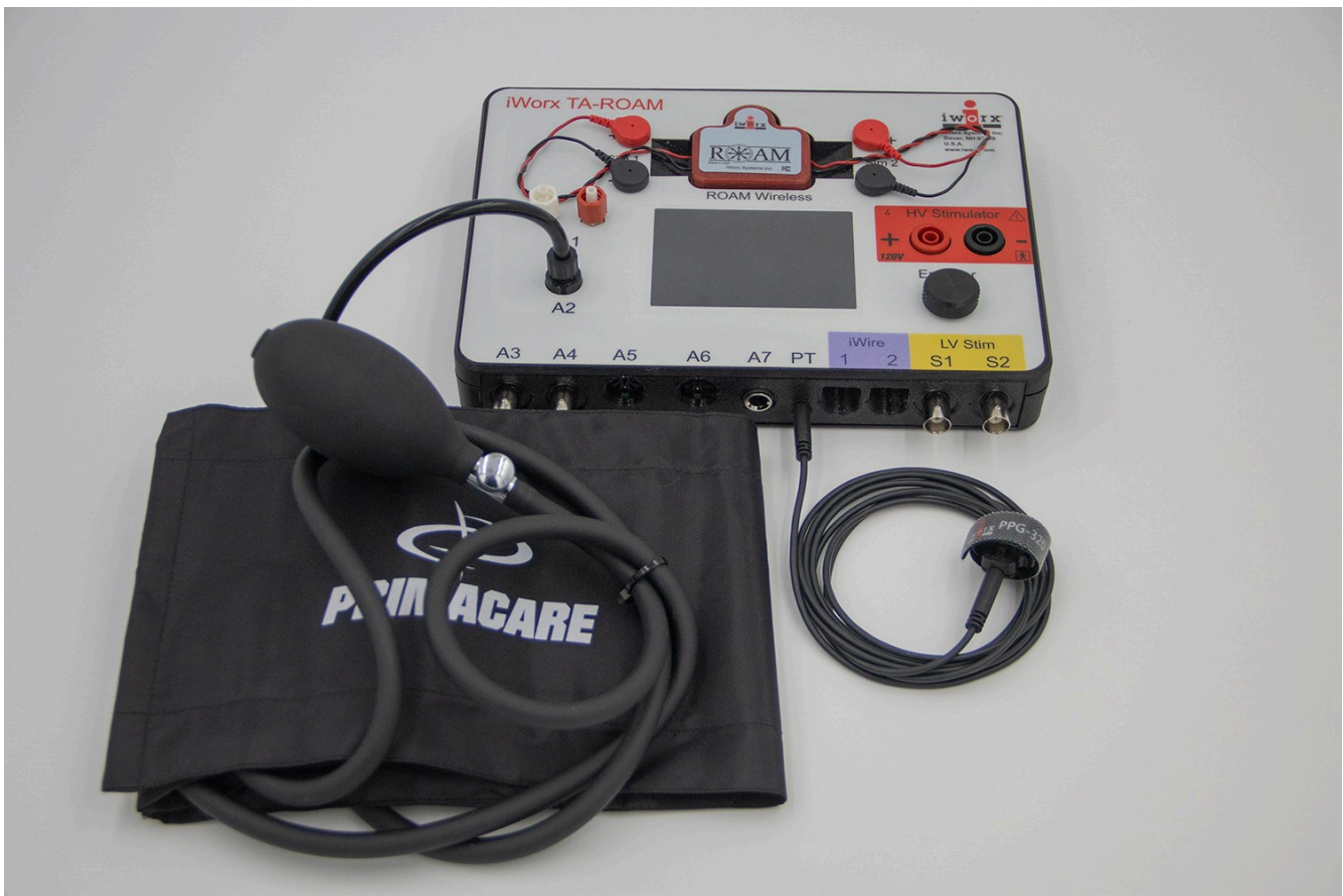
Figure HE-3-S2: The pulse oximeter and the BP-220 non-invasive blood pressure transducer connected to the TA.
