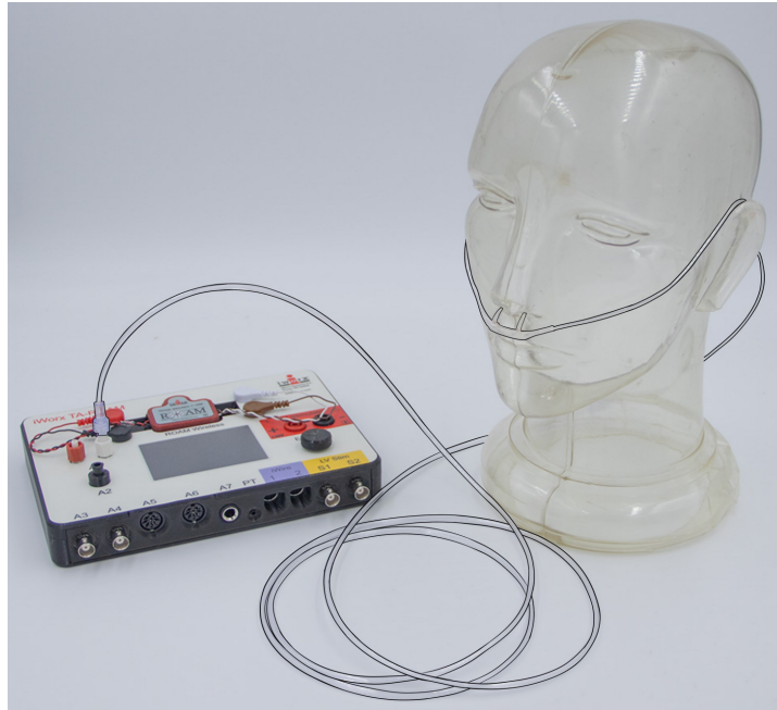
Figure HP-5-S1: Nasal cannula connected to the IX-TA and showing the proper positioning on the face.
