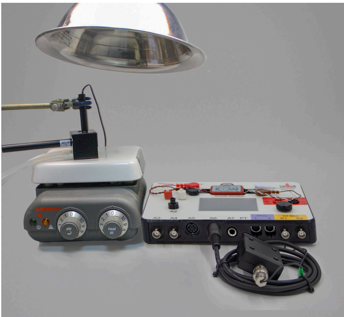
Figure CM-4-S2: The oxygen polarograph used to record photosynthetic electron transport. Black tape should cover the side of the polarograph block facing the light source, except on the area directly on the front of the chamber. The light is focused on this open area so that the circle of light is only large enough to cover the chamber.
