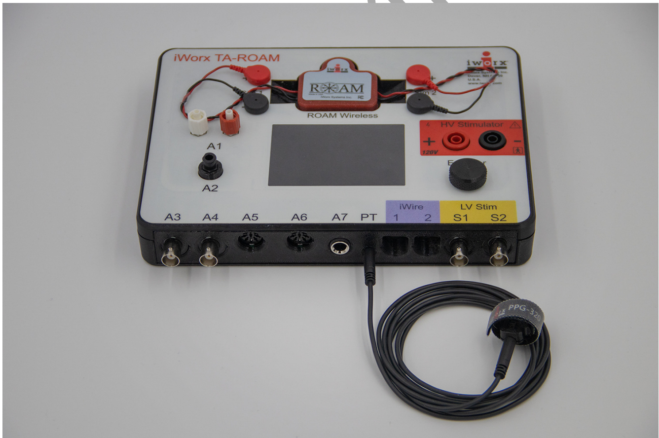
Figure HH-6-S1: The PPG-320 pulse sensor connected to the TA.
