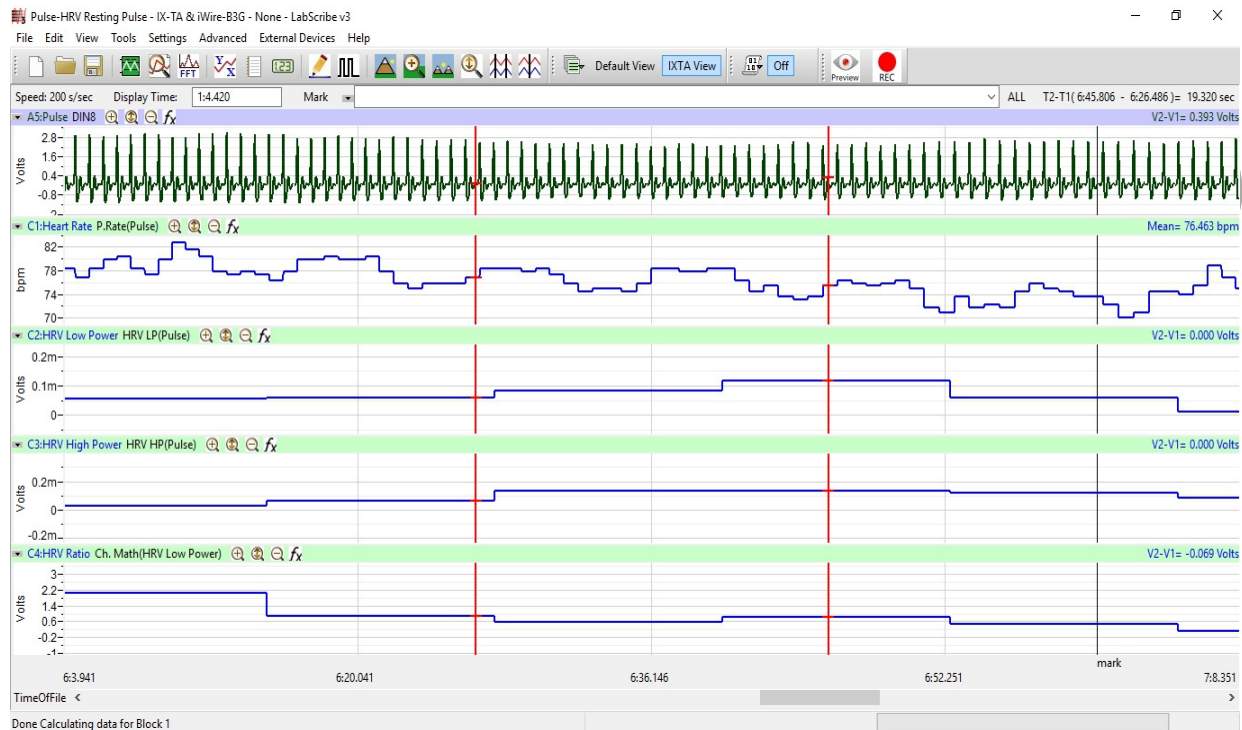
Figure HH-6-L1: The Pulse, heart rate, LP, HP, HRV ratio (from top to bottom) of a resting subject displayed in the Main window.
