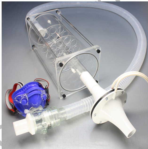
Figure HE-9-S6: The assembled devices used during metabolic studies. The assembly includes: the mixing chamber, smooth interior tubing, Nafion sampling tubing, flow head, spirometer, non-rebreathing valve, and mask.
