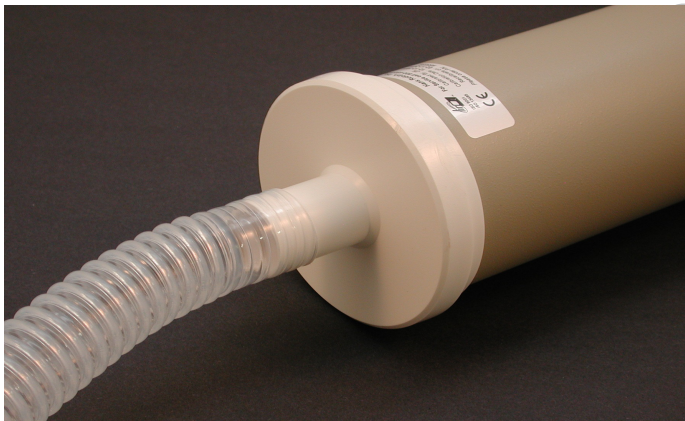
Figure HE-9-S18: 3 liter calibration syringe connected to the smooth bore tubing and Figure HE-9-S19: The smooth bore tubing connected to the mixing chamber.
