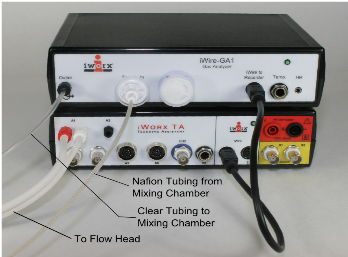
Figure HE-9-S4: The iWire-GA gas analyzer connected to an IXTA. All tubings are connect properly in this image.
