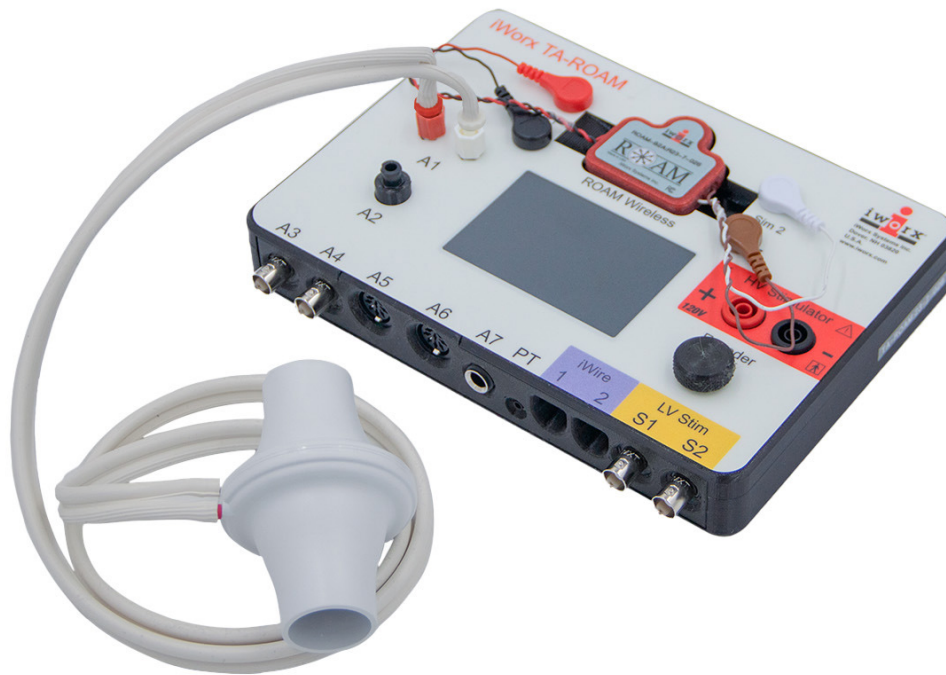
Figure HS-8-2: The flow head connected to the internal spirometer of the IXTA unit.
