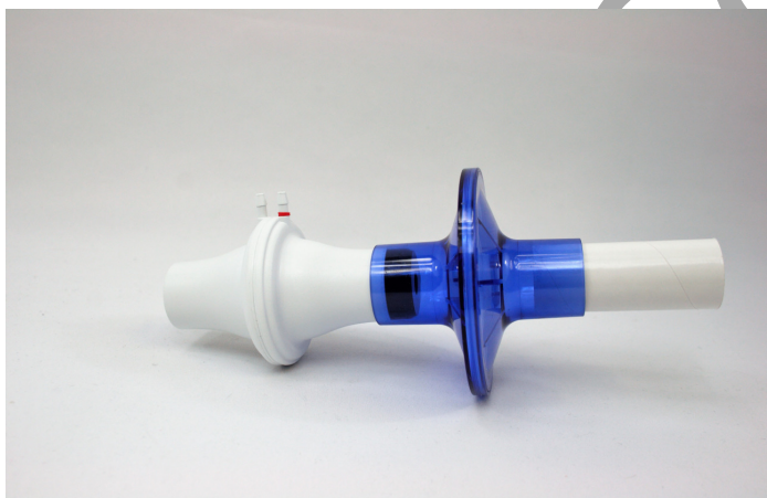
Figure HS-8-1: The A-FH-300 flow head and the airflow tubing, student respiratory kit with the spiro cap.
