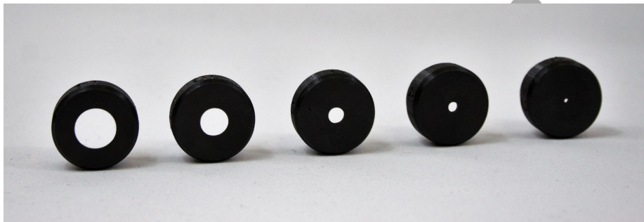
Figure HS-8-3: The 5 different size flow head caps for Restrictive experiment.
