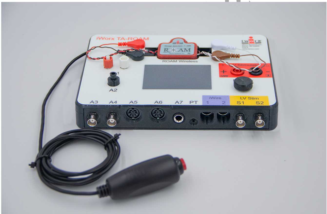
Figure HP-26-S2: The EM-220 Event Marker plugged into the EM1 port on the TA.
