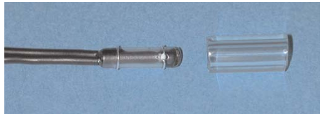
Figure 1: The A-SE-100 sleeve electrode probe (left) and the sleeve (right).
