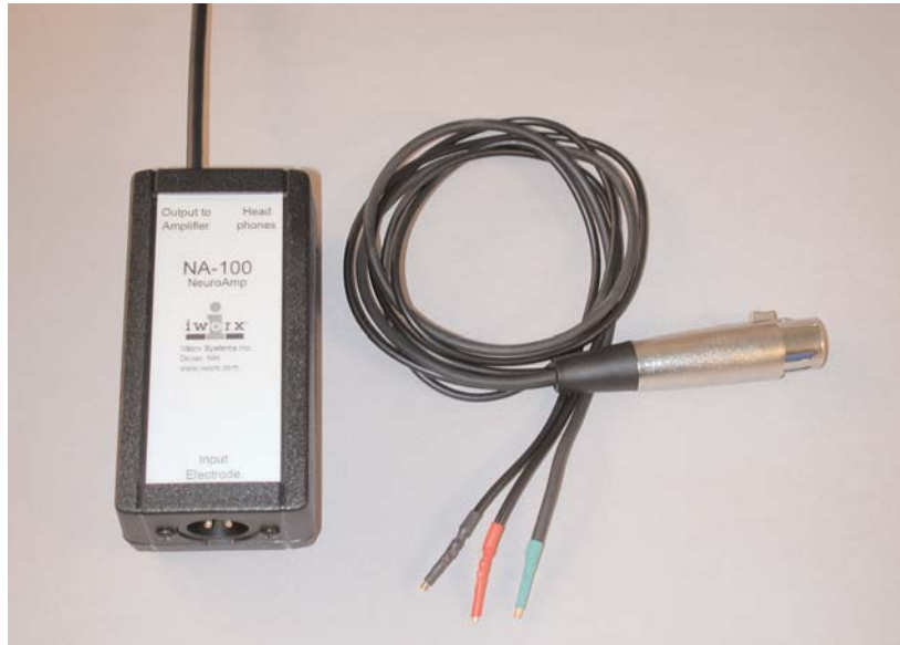
Figure 1: NA-100 Neuroamp Extracellular Amplifier and shielded input cable.
