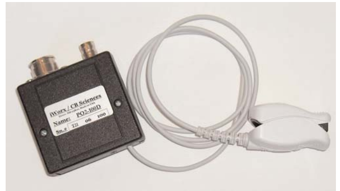
Figure 1: PO2-100D Pulse Oximeter and Plethysmography Sensor
