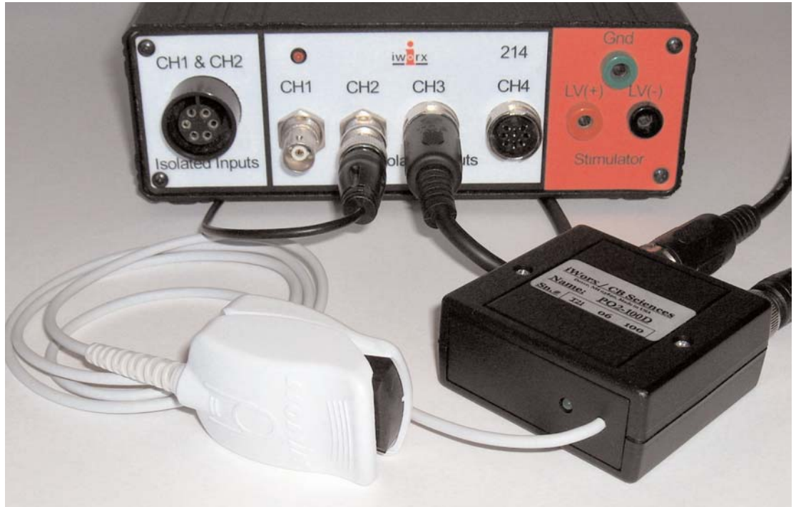
Figure 2: The PO2-100D Pulse Oximeter connected to Channels 2 and 3 of an IX/214 data acquisition unit.
