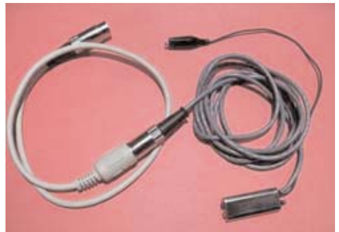
Figure 2: A DHS-300 Differential Head Stage Amplifier connected to a C-DIN-M/F gain cable.
