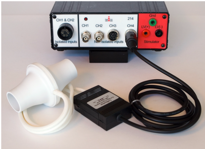
Figure 37A-2: A SP-304 spirometer connected to an IWX/214 unit.
