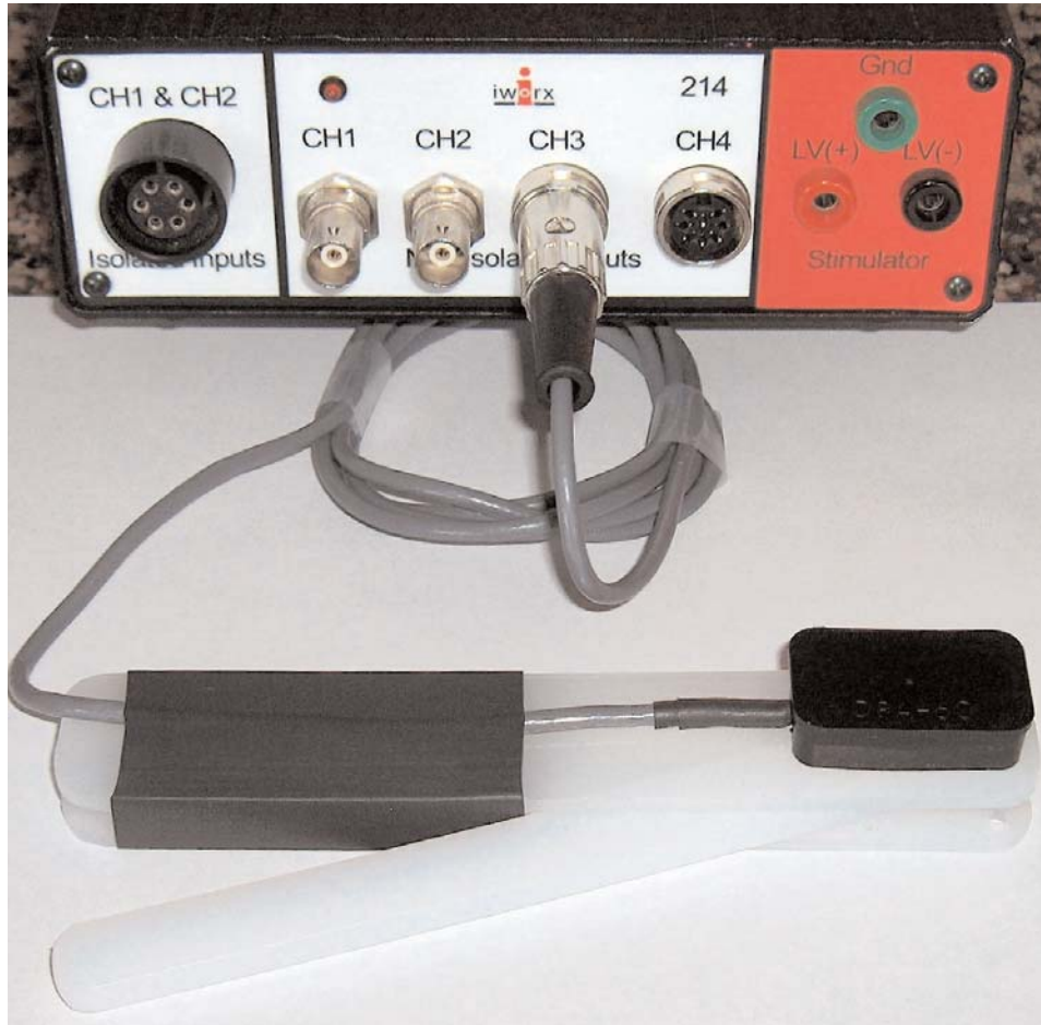
Figure 2: The GN-100 Single-Axis Goniometer connected to an iWorx 214 Recorder.
