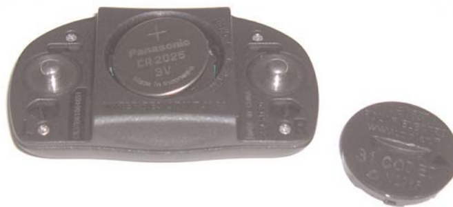
Figure 3: The HRB-100 heart rate transmitter with the battery compartment open, showing the proper orientation of the battery.
