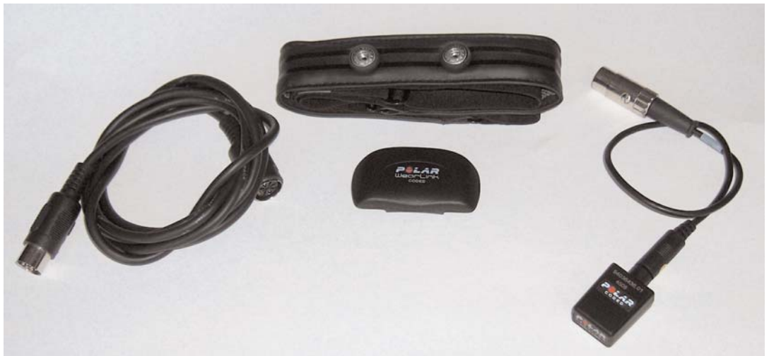
Figure 1: The components of the PHRM-100 Polar heart rate monitor, from left to right: the DIN8 extension cable; the HRB-100 transmitter and its sensor band; and, the HRR-100 receiver with its DIN8 adapter.
