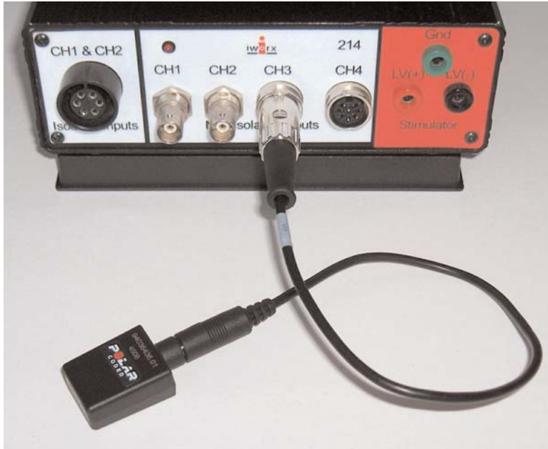
Figure 2: The HRR-100 heart rate receiver connected to the DIN8 input of an iWorx 214 data recorder.
