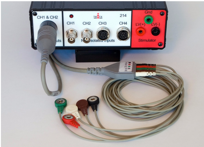
Figure HM-7-4: A five lead EMG cable connected to an IWX/214.
