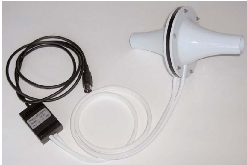
Figure 2: The A-FH-1000 Flow Head from the GAK-100 kit connected to the SP-304 Spirometer with a pair of airflow tubes.
