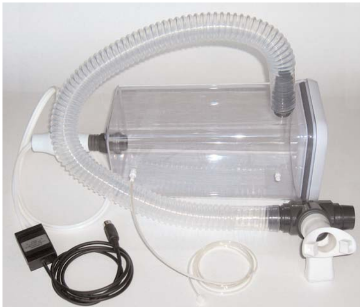
Figure 4: The spirometer circuit used to measure the volume of air exhaled by the subject, and provide oxygen and carbon dioxide samples from the exhaled air to the gas analyzer.
