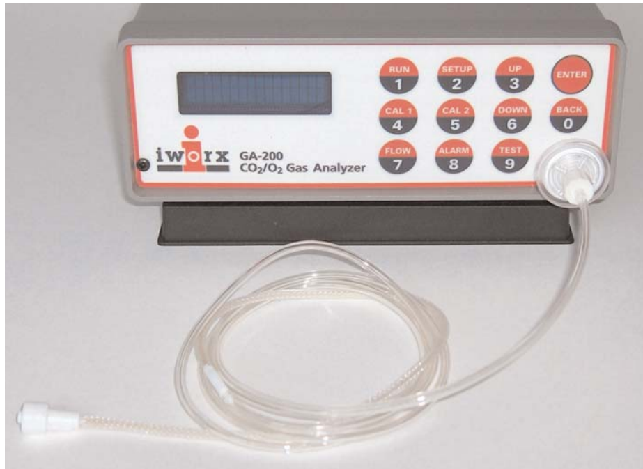
Figure 5: The front panel of the GA-200 gas analyzer showing the filter and Nafion sampling tubing connected to its inlet.
