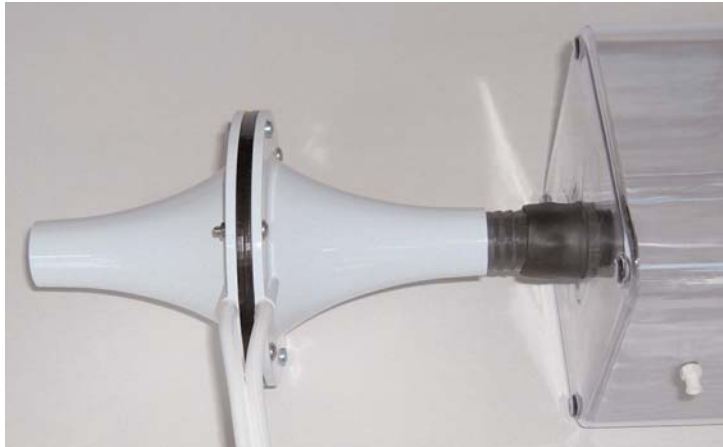
Figure 3: The inlet of the A-FH-1000 Flow Head attached to the outlet of the mixing chamber.
