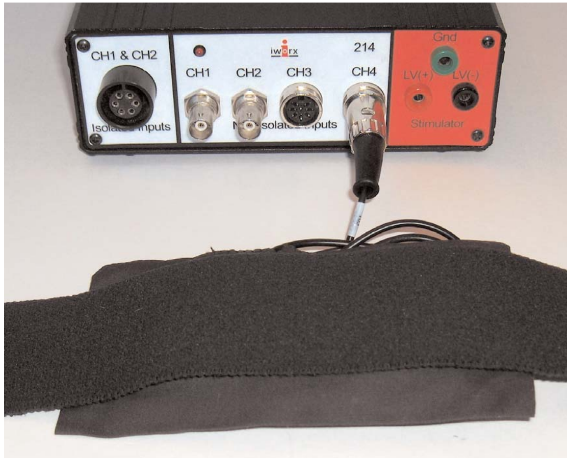
Figure 2: The RM-204 connected to Channel 4 of an IWX/214 data acquisition unit.
