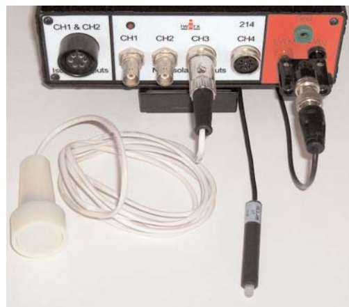
Figure 2: The male double banana-female BNC adapter.
