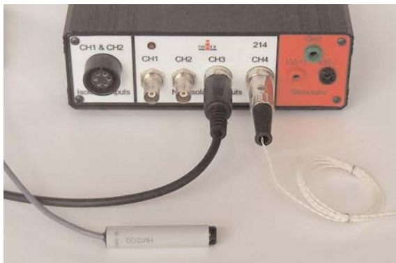
Figure 2: The HS-100 Humidity Sensor connected to an iWorx/214, along with a TM-100 Temperature Sensor.
