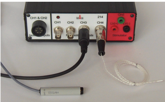
Figure HS-100-3: The HS-100 humidity sensor and the TM-100 temperature sensor connected to an IWX/214
