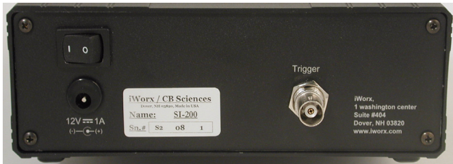
Figure SI-200-2: The rear panel of the SI-200 showing the BNC Trigger input on the right, and the power switch and receptacle on the left.
