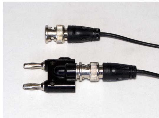
Figure SI-200-4: BNC-BNC cable attached to a BNC-Double Banana adapter. The tab on the side of the adapter identifies the prong that is connected to the ground jack.
