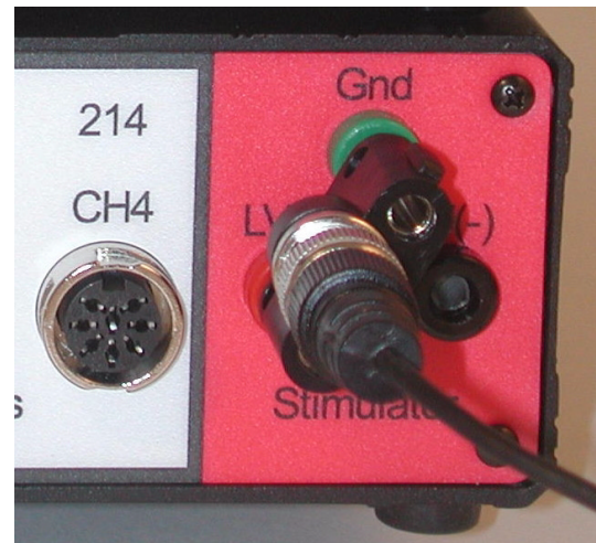
Figure SI-200-5: The BNC-double banana adapter and BNC-BNC cable connected to the stimulator output of an IWX/214.
